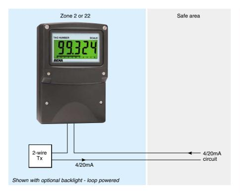
The BA324NE loop powered 4/20mA indicator is a fourth generation field mounting instrument that is mechanically compatible and electrically similar to the earlier BA324ND. It has a much larger full 5 digit display and guaranteed performance between -40 and +70°C. Like it's predecessor, the BA324NE is housed in a robust IP66 enclosure with a separate terminal compartment.
